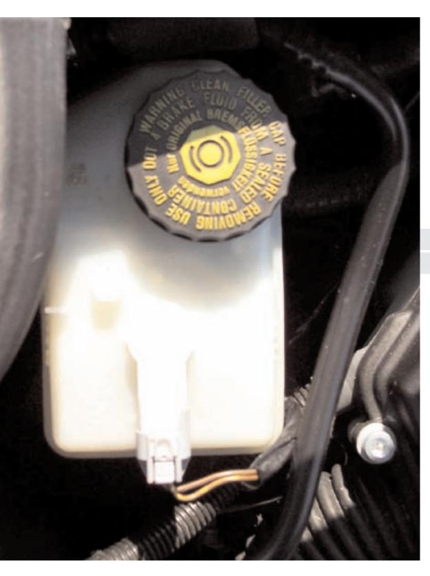
Maintenance - changing old brake fluid removes the absorbed water from the brake system. Water compresses at a different rate than the dry brake fluid, so squeezing the brakes on going into turn 1 with old fluid can feel a little squishy. Old brake fluid must be flushed out or water absorbed by the fluid eventually causes internal rust on the disk calipers and pistons.
