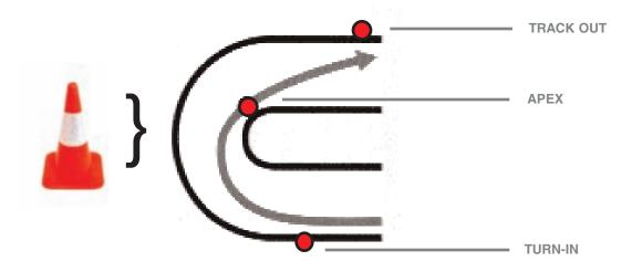
Anatomy of a corner: Shown above is a basic 90° right-hand corner and a late apex radius through it. There are three basic components to each corner, each usually marked with an orange cone.
