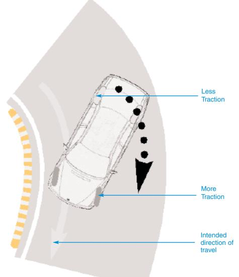
Oversteer: The rear tires have less traction than the front tires, and the back end of the car begins to slide. The car has turned more than you want it to, so it has oversteered. This is also called "being loose," or "fishtailing."
