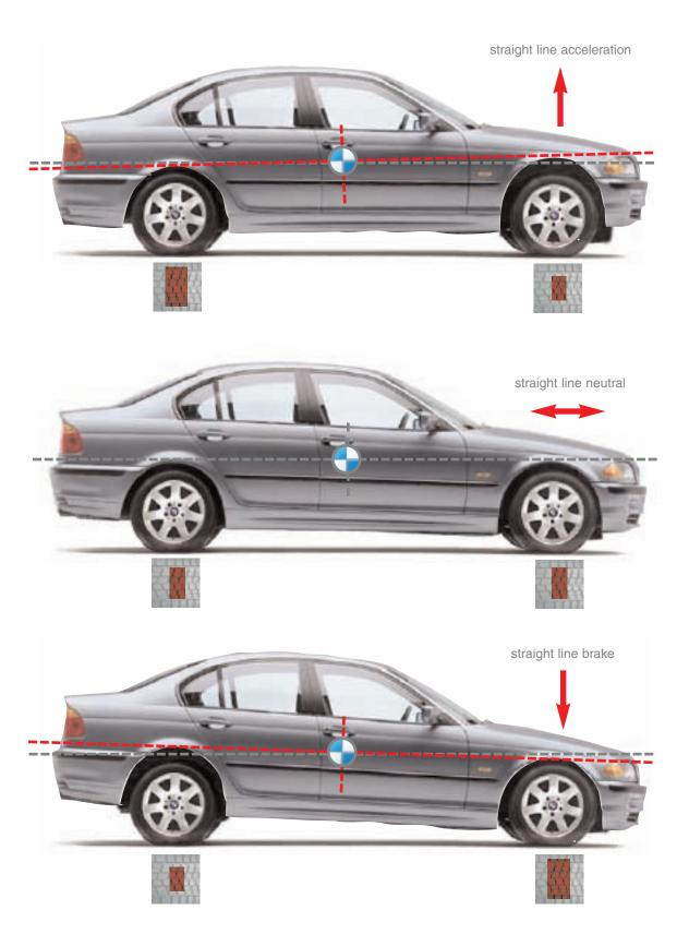
Weight Distribution: Much of your time on the track will be spent managing the cars weight, or better stated, intentionally shifting the weight in a controled and smooth manner to the location where it will do the most good. You are connected to the track by your tire's contact patch, an area not much larger than the palm of your hand, or the ball of your foot.
