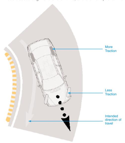
Understeer: The front tires have less traction than the rear tires, and regardless of the steering corrections, the car continues to "plow" or "push" straight ahead. The car does not steer as much as you want, so it is understeering. Understeering in effect, increases the radius of a turn.
