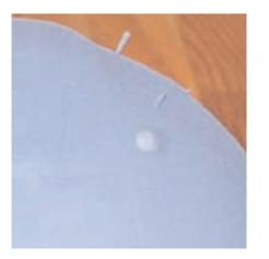
.04 Prime the shell in several thin coats allowing dry time between, and lightly re-sand.
