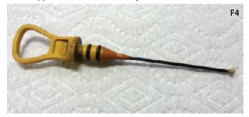
before it broke apart. How many of you have broken the \$2 dipstick on a '55 Chevy? The \$30 MINI dipstick made of exotic materials breaks. I am at a loss to explain how this can happen and it's no wonder that newer MINIs have also eliminated a stick with some lines scribed on it in favor of coaxial capacitors and a black box.
