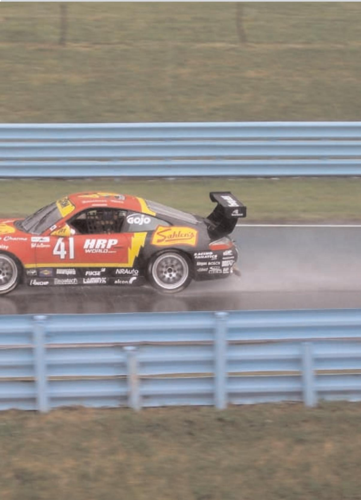
“Keep in mind that adjusting tire pressures is a small thing you might be tempted to take too far. On stock suspensions, there is not going to be sufficient negative camber to prevent a tire from rolling onto its sidewall under cornering. For example, on a track with primarily right-hand turns, the left front tire will tend to roll onto its sidewall no matter how high tire pressure is raised. So don't overinflate. This is where common sense and seat of the pants tuning become important too.”
