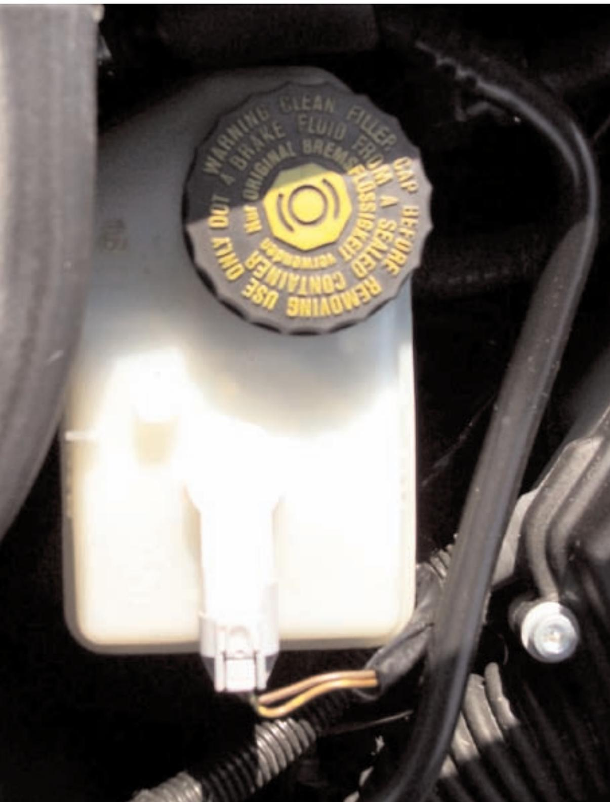
**Maintenance** - changing old brake fluid removes the absorbed water from the brake system. Water compresses at a different rate than the dry brake fluid, so squeezing the brakes on going into turn 1 with old fluid can feel a little squishy. Old brake fluid must be flushed out or water absorbed by the fluid eventually causes internal rust on the disk calipers and pistons.
