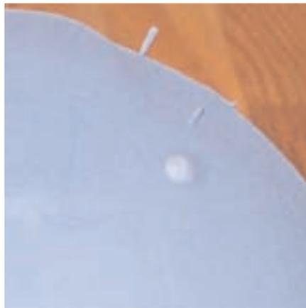
**.04** Prime the shell in several thin coats allowing dry time between, and lightly re-sand.
