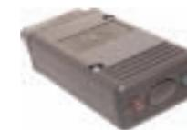
The shark provides an increase in the factory rev-limit, re-maps the throttle, fuel and spark, as well as the acceleration enrichment, transition fueling and VANOS control as needed to optimize the vehicle for operation on premium fuel on all OBD II 6 Cylinder BMWs.
